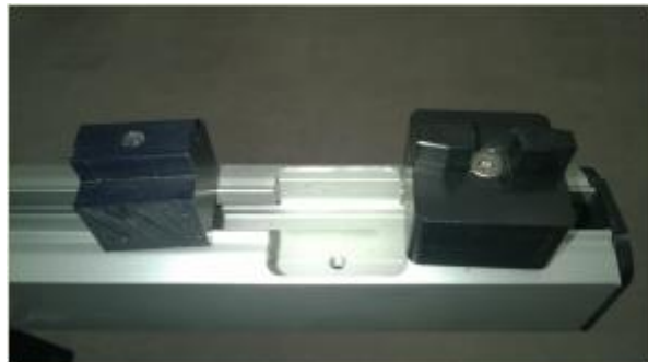
PVC black and stop block removed from bottom track.
