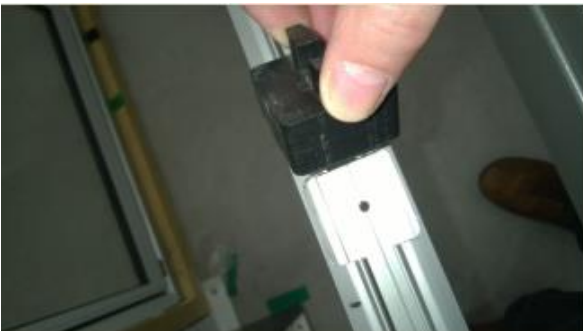
Removing PVC Block from bottom track.
