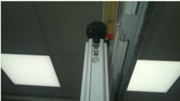
Lead panel locking lever on pivot wheel
